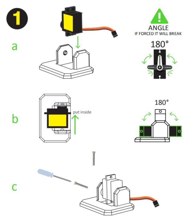
Put the micro servo inside feet and then push it inside, if is to hard maybe need to clean more the area with a cutter. Is very important to check that the servo is able to rotate at 180 degrees to each side.
