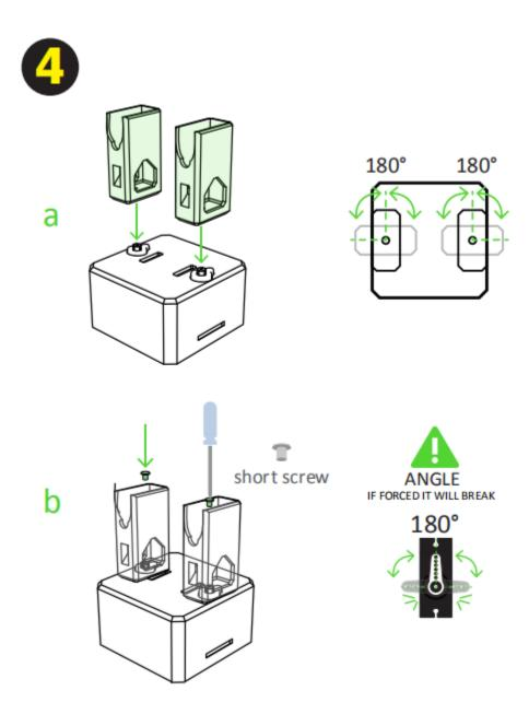
Connect the legs to the hub of the micro servo, important like the foot servos, you must check the legs are able to rotate 180 degrees each side respect to the body.
