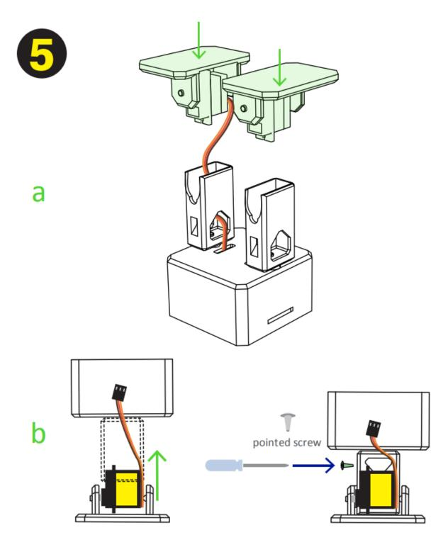
Taking care of the cables as showed in the illustration, you should put the cables inside the slots of the body passing through the hole of the legs.
