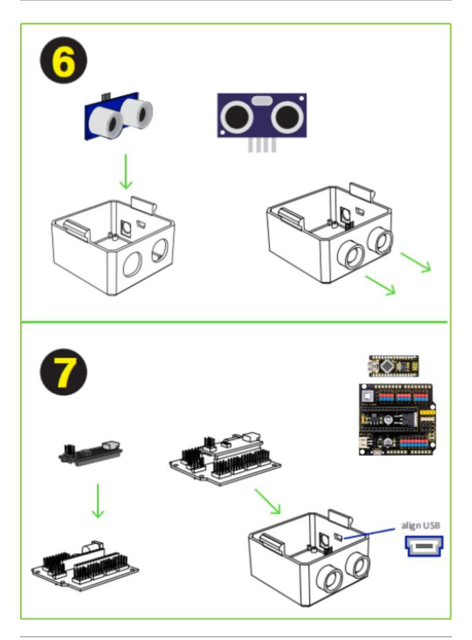
Start from the ultrasound sensor is important to pull out the eyes to the limit. Then put the Arduino nano in the shield, optionally you can weld the positive cable of battery holder to Vin in the board and negative cable to any GND.
