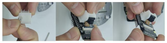
Step 7: Plug the ESP32-CAM development board into the car motor driver board, then the video car is successfully assembled.
